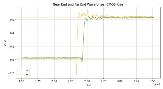
$$Z_{PUN} = \frac{50\Omega v_{out}}{v_{A}} - 50\Omega = \frac{50\Omega 1.8V}{0.64V} - 50\Omega = 91\Omega$$
