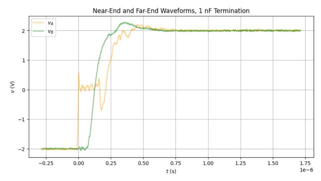
The trace is consistent with our expectations: RC charging pattern at far-end, which is propagated back to the near end. The near-end waveform didn't fully drop to 0 due to the opposite reflected wave from far-end. This is because the capacitor wasn't an ideal short when charged by a pulse with a finite slew reate.
