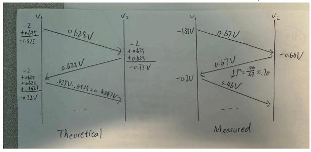
Theoretically, the initial  $v_1^+$  step should have  $2*2V\frac{50}{50+220+50}=0.625V$ , which is fully reflected at the far end, and then reflected at the near-end at a coefficient of 0.6875, propagating back and forth until equilibrium.
