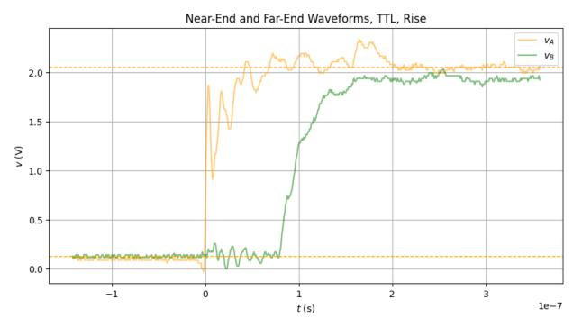
From the 74F04 datasheet,  $V_{\text{high}}$  goes to 0.9  $V_{\text{CC}}$  = 3.6 V.
