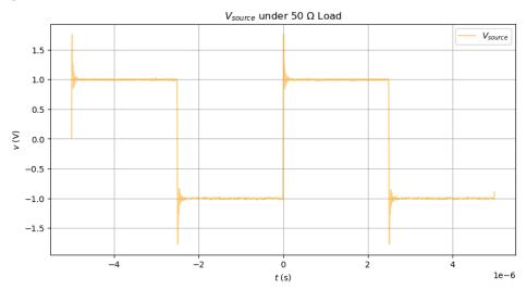
Steady-state  $V_{\text{source}}$  measured is about  $\frac{1V}{V}$ . The simple circuit is a voltage divider, which suggests a matched source resistance to split half source voltage amplitude  $\frac{1V}{2V} = \frac{R_c}{50\Omega + R_c}$ .
