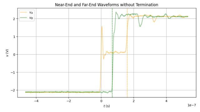
When the input square wave switches phase from -2V to +2V, the pulse has magnitude of +4V However, v<sub>A</sub> initially only experiences a 2 pulse, suggesting that the rest are divided by the line's characteristic impedance.
