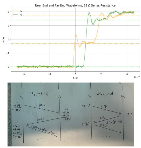
Same analysis here. The measured  $\Gamma = \frac{0.3V}{1.7V} \approx 0.176$ , pretty close to the calculated values.
