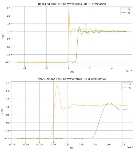
Compared to Q2, although the initial near-end pulse remains the same, the incident wave does reflect back at the far end, halfing the overall change. The result is also consistent with the voltage division at the termination, that the termination resistor divides half the voltage with the source impedance.
