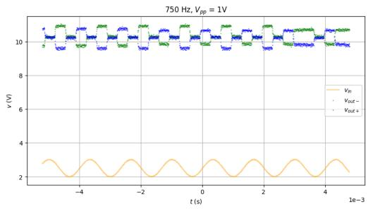
Because our DAC has amplification issues, we used the DAC from Charlie and Millie after they were done, and took separate measurements with the regular 10k output loads.
