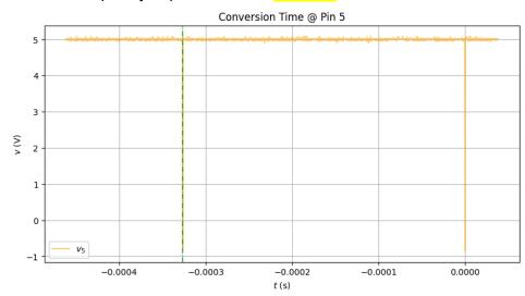
We observed the period between two peaks at pin 5 (INTR), signaling conversions.
