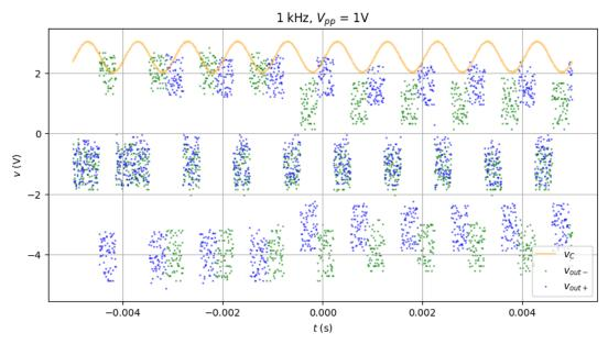
Theoretically, we should be able to recover the signal with ADC/DAC up to a bandwidth of 1.53 kHz. However, due to nonideality (white Gaussian noise for example), the upper limit of the bandwidth of the recoverable signal is much smaller than expected.
