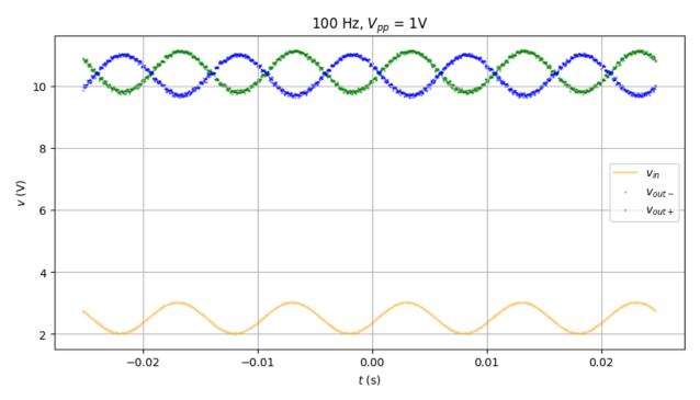
As the digital input at DATA increases,  $I_{out^+}$  increases while  $I_{out^-}$  decreases. An increasing output current will pull down the output voltages. Therefore,  $V_{out^+}$  (blue) has an inverting phase, while  $V_{out^-}$  (green)'s phase is not inverted.
