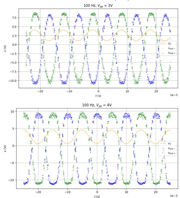
As the input amplitude increases, the output voltage swing rises proportionally. The output waveform looks fine at  $V_{pp}$  = 3V at input, but distorted at  $V_{pp}$  = 4 V. This is because inside, the DAC transistor output voltage swing is reached. Beyond that, the transistors will no longer be in the active mode. Therefore, the outputs are capped.
