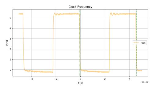
$f = 1/(t_2 - t_1) = 1/(4.55e-6 s - 6e-8 s) = 223 kHz$ The clock frequency at pin 19 is about 223 kHz.
