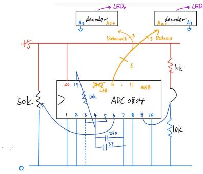
Below are the results. The input ranges from [0, 5], and the octal output ranges from  $[0, 63_{10}]$ . Therefore,  $V_{out} = LED_{10} * 5/63$
