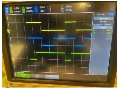
Channel 1 (yellow) is Q as the output. Channel 2 (green) is R. Channel 3 (blue) is S.
