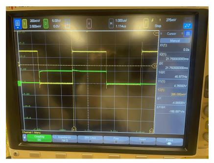
Waveforms at 1 kHz. Channel 1 (yellow) is the input. Channel 2 (green) is the output.
