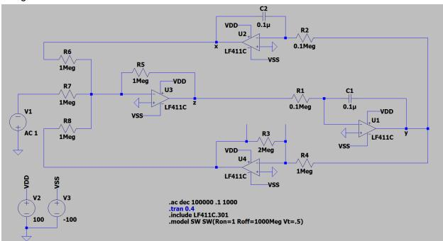
Since the frequency increases 100 times, I ran the transient simulation for 0.4 s instead of 40 s.
