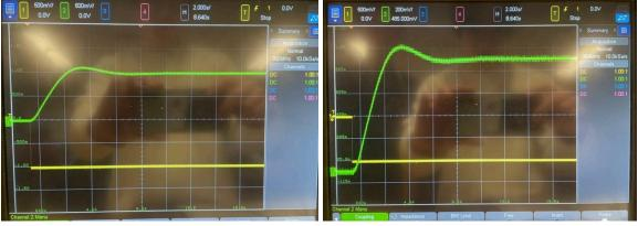
They match perfectly with the theoretical and simulated behavior, with an overshooting peak at about 4s, followed by damped oscillation.
