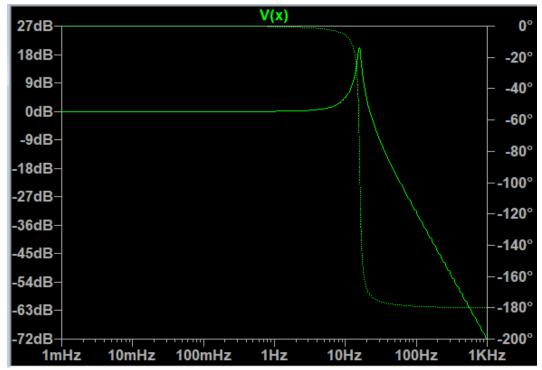
There is a sharp peak of high gain at a resonant frequency of 100 rad/s. The phase shift is also sharper around resonance.
