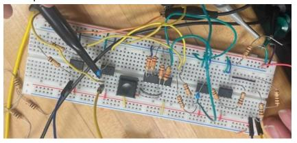
We used a CMOS switch array to ground the output of U2 and U4 to satisfy the initial conditions x(0) = 0 and x'(0) = 0.
