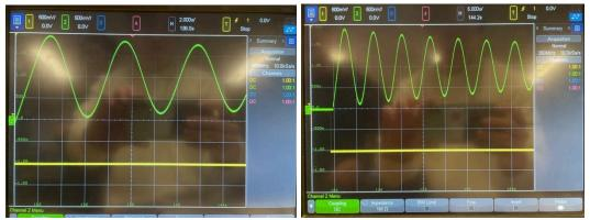
The amplitude of the first cycle was around 1V, which matched the simulated response. However, the response began to slightly decay afterward. Still, the sinusoidal oscillation was still visible after 40 seconds.
