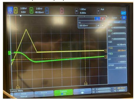
The output voltage at t = 7 s is -1.4 V, which maps to  $\frac{280 \text{ ft/s}}{\text{s}}$ .
