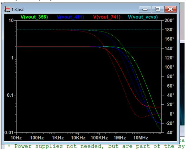
Among the commercial models, LF356 (green) has the widest frequency response, up to about 1 MHz, until the gain declines significantly below 2.
