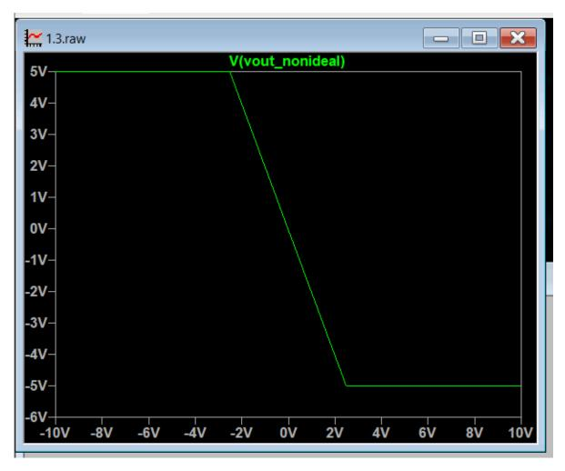
vout saturates at 5 V and -5 V due to the arctangent function.
