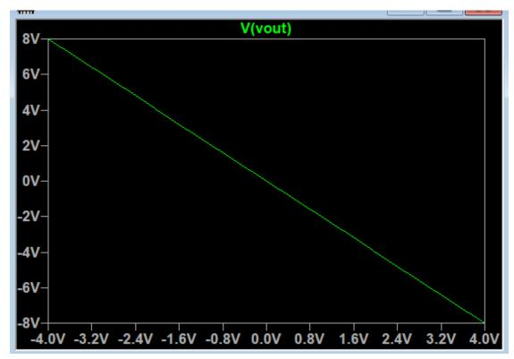
vout vs vin: The slope -2 is the VCVS's gain.
