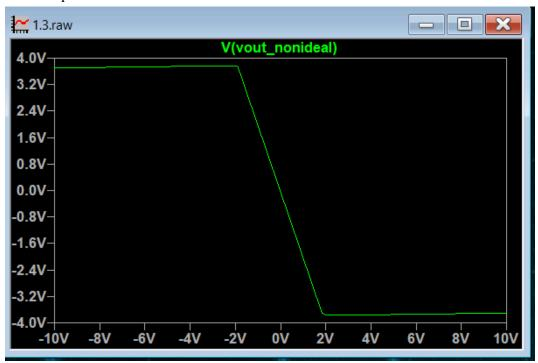
From the DC sweep curve, the output range is approximately -3.7 V to 3.7 V. The curve has sharp corners, very ideal.
