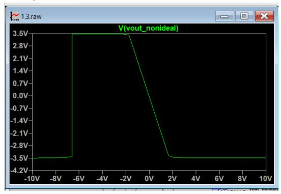
The output range is approximately -3.5 V to 3.5 V. The corners are round, so there is some distortion before saturation. 1 V is in the linear region, so this does not affect our gain.
