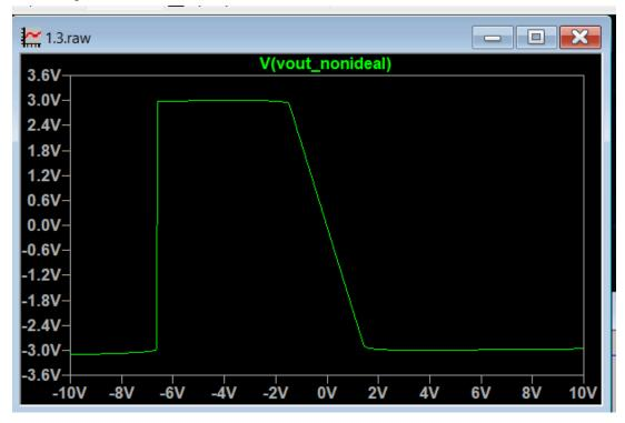
The output range is approximately -3 V to 3 V. Similar to LF411C, the corners are not sharp before saturation.
