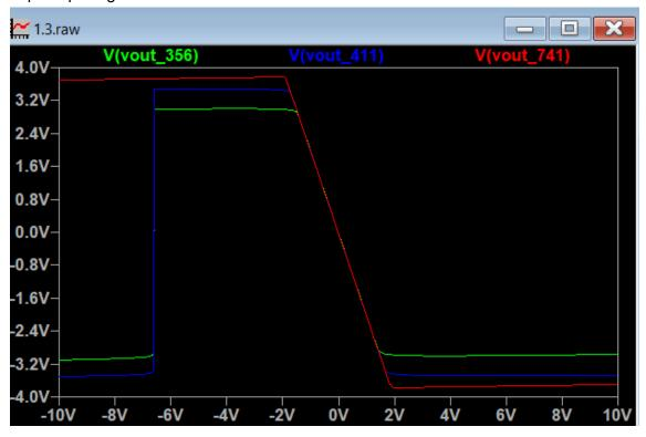
In terms of output voltage vout\_nonideal in the circuits above, LF411C's output is the closest to ideal, at 99.997% of the ideal gain.
