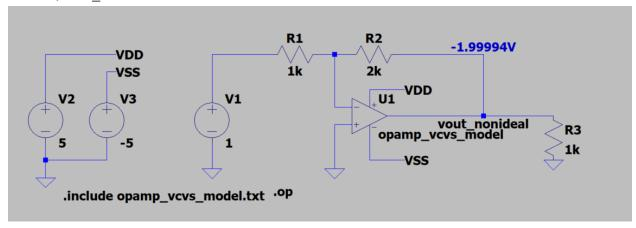
The calculation matches the simulation result exactly.
