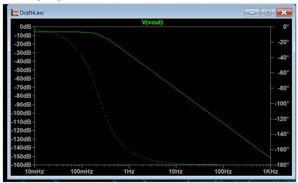
The solid trace is the gain, and the dashed trace is the phase shift.
