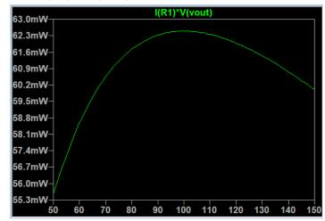
The shape is an upside-down curve, with a maximum at  $R_{\rm load}=100\Omega$ . If  $R_{\rm load}$  is too low, most voltage will be wasted by  $R_2$ . If  $R_{\rm load}$  is too high, less current will pass through the series circuit, decreasing the power. Since power is the product of voltage and current, the curve is bell-shaped, with a maximum occurring when  $R_{\rm load}=R_2$ .
