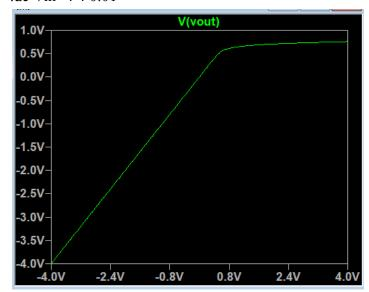
At approximately Vin < 0.6 V, Vout = Vin. Once Vin > 0.6 V, Vout caps at 0.6 V. Therefore, the transfer curve is initially linear but flattens for positive Vin.
