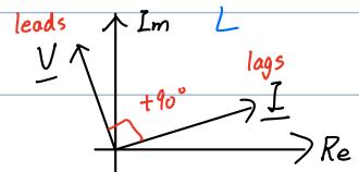
Impedance  $\underline{Z} = I_m \angle \phi_I, \underline{V} = V_m \angle \phi_V \quad \underline{Z} \equiv \frac{\underline{V}}{\underline{I}}$
