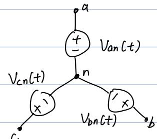
$$\checkmark V_{an} + V_{bn} + V_{cn} = 0 \rightarrow \sum \text{ in } t \text{ also } 0.$$
