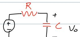
$$M(w) = \frac{1}{\sqrt{1 + (\frac{w}{w_c})^2}} \quad \frac{1}{\sqrt{2}} \text{ at } w_c \quad , \quad \phi(w) = -\tan^{-1} \frac{w}{w_c} \rightarrow -90^\circ$$
