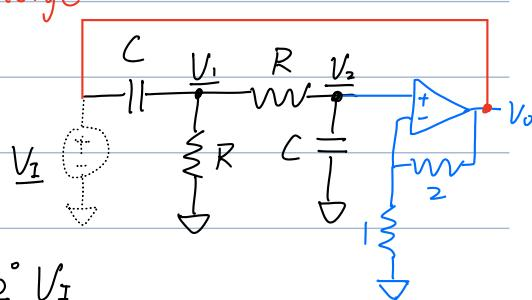
Then use n.i.amp to amplify back 3x.  $\rightarrow$  feedback as  $\underline{V}_2$ , self-driven
