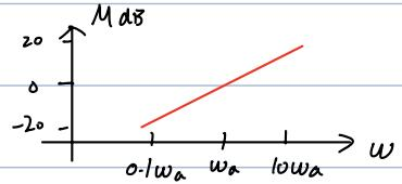
$$3. 1 + j \frac{w}{w_a} \approx 1, \quad w \ll w_a \quad \left. \begin{array}{l} \text{straight line approx. of 1 and 2.} \\ 3 \text{ dB at } w_a \end{array} \right\}$$
