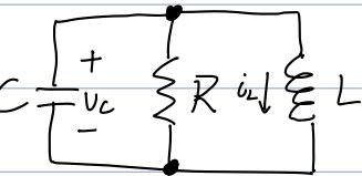
$\text{④} \Rightarrow \text{② } C V_C(0) + \frac{V_0}{R} + I_0 = 0$
